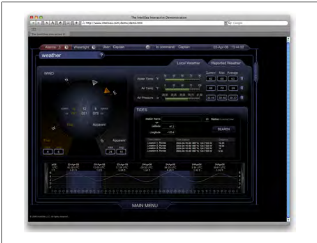
Figure 2-10. The IntelliSea yacht alarm, monitoring, and control system
