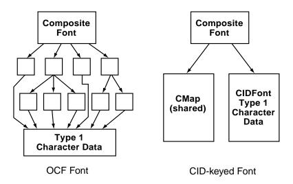
Figure 1 The structure of OCF and CID-keyed fonts
