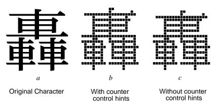
Figure 4 Effect of rendering with, and without, Counter Control hints
