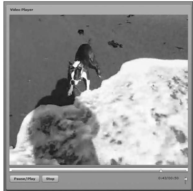
Figure 10-12. The playback progress is being displayed by the HSlider component added under the progress bar.
