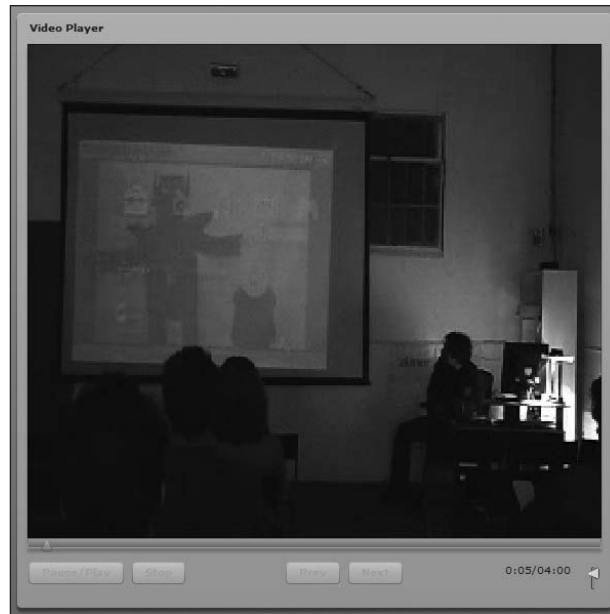
Figure 10-17. All controls except the volume slider have been disabled, because this video is designated as an “ad” by the type attribute in the playlist.xml.
