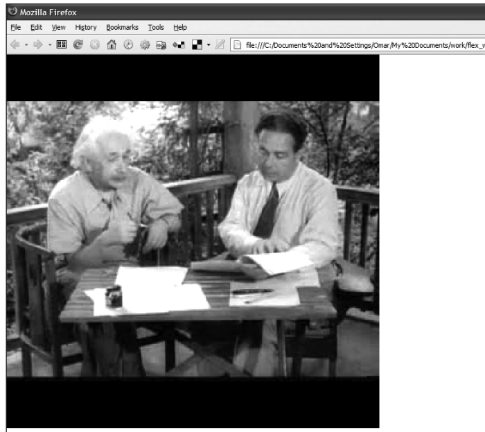
Figure 10-4. The property maintainAspectRatio causes the video to scale and keep proportion, resulting in the black strips.
