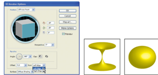
The 3D Revolve Options dialog box, the results of the Revolve effect with Left Edge selected, and the results of Revolve with Right Edge selected.
