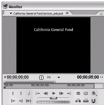
Figure 7: Choosing the Document Size option imports the layer using the entire Photoshop document's pixel dimensions. This makes it easy to reassemble the layers as they appeared in the Photoshop document.
