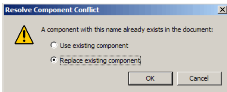
Figure 9. Select the option to Replace existing component in the Resolve Component Conflict dialog box
