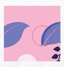
Misalignment of color planes can be an issue in industrial inkjet applications, caused by many of the same factors found in commercial offset and flexo print shops, e.g. the side-to-side movement in any roll-fed, web press. But there are also a few inkjetspecific causes of potential misregistration, and alignment issues may be exacerbated by nozzle configuration within the inkjet array.
