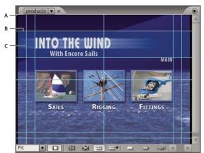
Menu with guides displayed A. Zero point of menu B. Horizontal guide C. Vertical guide
